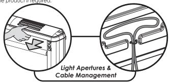
To maximise the effectiveness of Halo Shades in catching flying insects, the top of the product has light apertures to increase the UV irradiance emitted from the product. However, these apertures can be covered to protect the glueboard from debris and prolong its life, by simply sliding the reflective aluminium cover forward.
