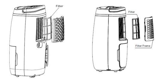
The standard dust filter can be replaced by a HEPA filter for better air cleaning and to remove more particles from the air.
