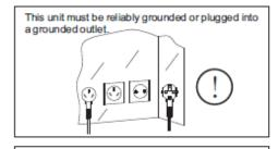
This unit use special electrical connection and outlet, don't use other extension wire or portable outlet.
