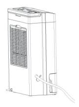
If you find that the water is flowing back into the tank but the hose is running perfectly downhill with none of the above problems then make a 4mm diameter hole in the top of the hose 30mm from the dehumidifier to allow air into the top of the hose and to balance out the air pressure imbalance that is stopping the water from flowing.
