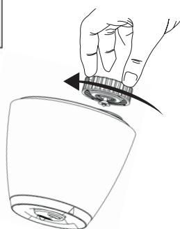
4. Close the tank lid, turning it to the right. It is important to FIRMLY secure cap after filling the tank with water.
