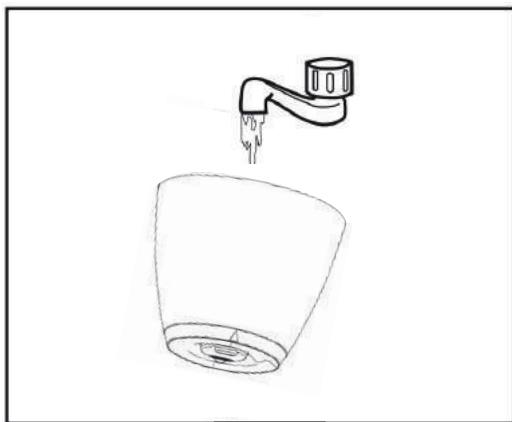
3. Pour cool, clean water directly into the tank. Do not pour anything but water into the tank.
