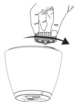
2. Flip over water tank and open the tank lid, turning it to the left.
